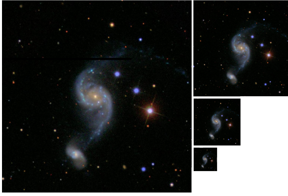
Figure 4: Four decreasing level-of-detail versions of a sky image tile (for demonstration purposes, an SDSS image). As the user zooms further out from a source less details are needed to convey information. This image pyramid demonstrates this effect with four levels of resolution, starting with a 1024x1024 pixel image and going down to a 128x128 pixel image.
