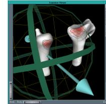
We have implemented a C++ and OpenInventor prototype of our visualization technique. The user can explode the joint for better viewing, disable or enable contour and distance viewing, and remove bones from the joint.
